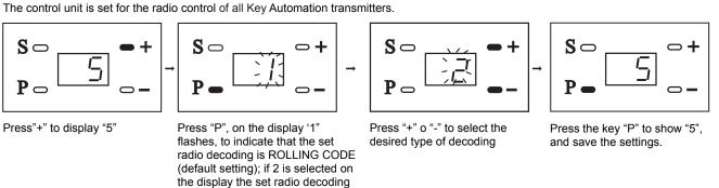
Note: in order to exit the programming and save the parameters push P button for 5 seconds.
